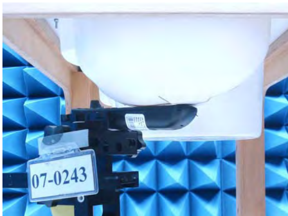
Figure 17. Left Head SAR Test Setup (Cheek)
