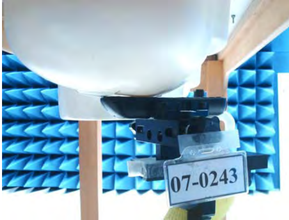
Figure 15. Right Head SAR Test Setup (Cheek)
