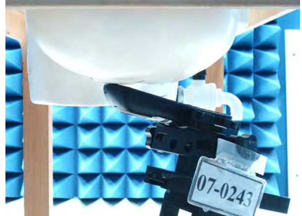
Figure 16. Right Head SAR Test Setup (Tilted)
