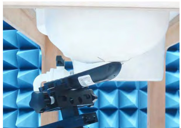
Figure 18. Left Head SAR Test Setup (Tilted)
