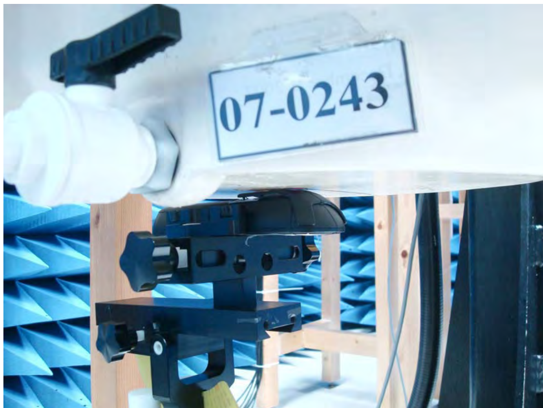
Figure 19. Body SAR Test Setup (Flat Section)
