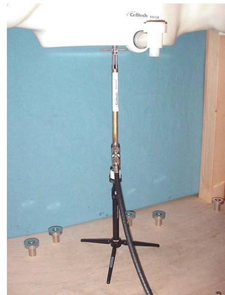
1900MHz Dipole Setup
