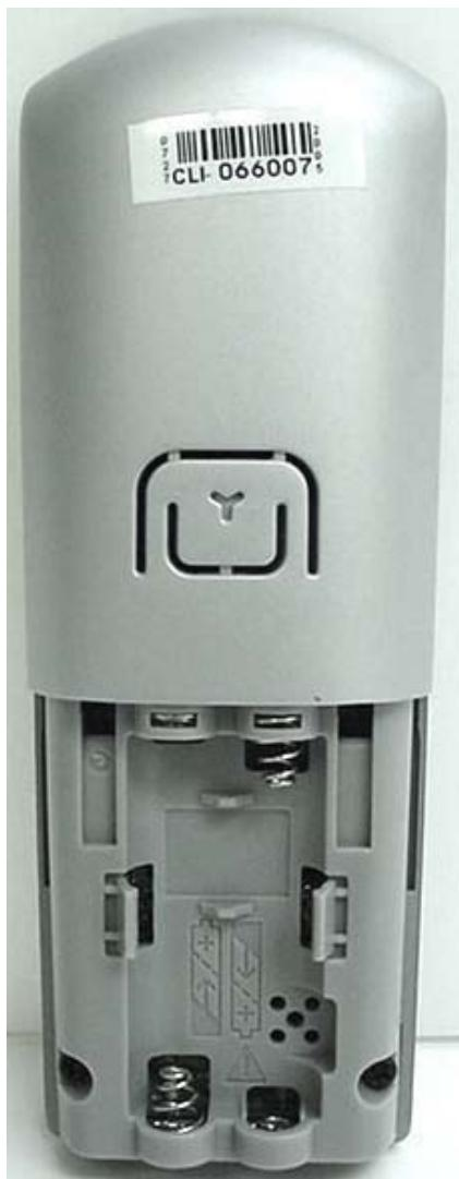
DUT Battery Compartment
