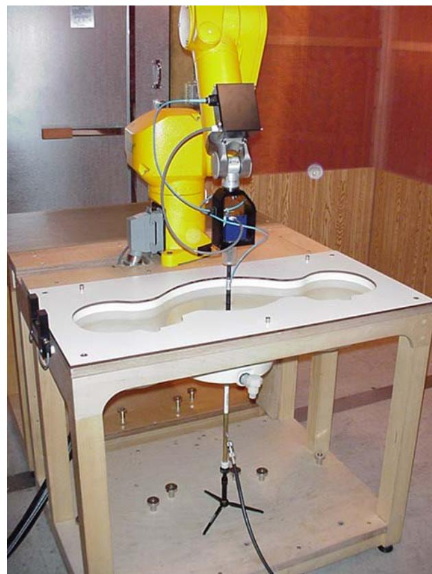
DASY4 Measurement System with SAM Phantom
