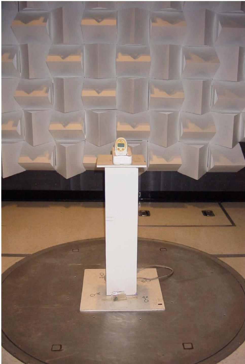
RADIATED EMISSIONS TEST SET UP (HANDSET) MODEL 08053R
