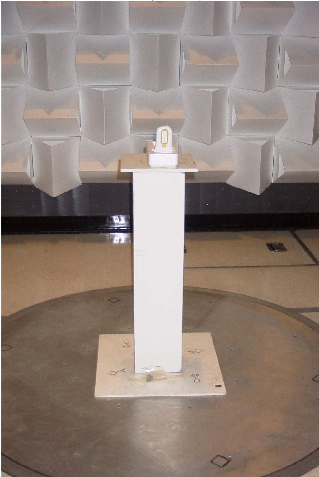
RADIATED TEST SET UP (HANDSET) MODEL SCD588R:
