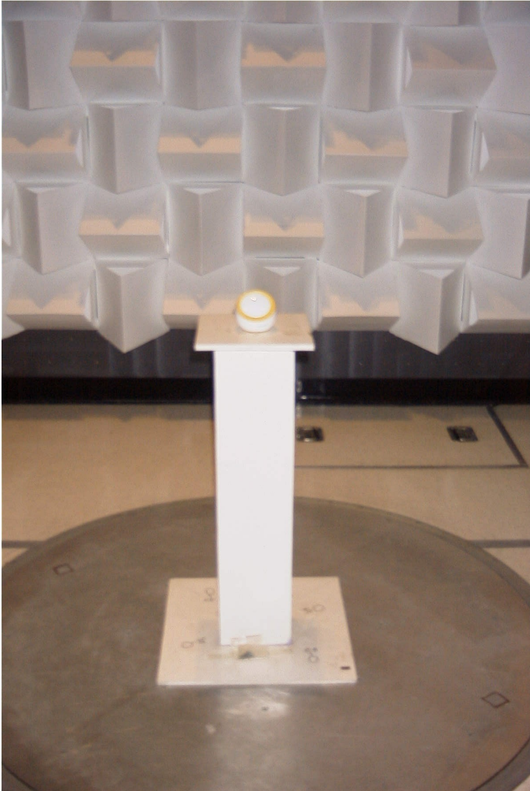
RADIATED TEST SET UP (BASE) – MODEL SCD587:
