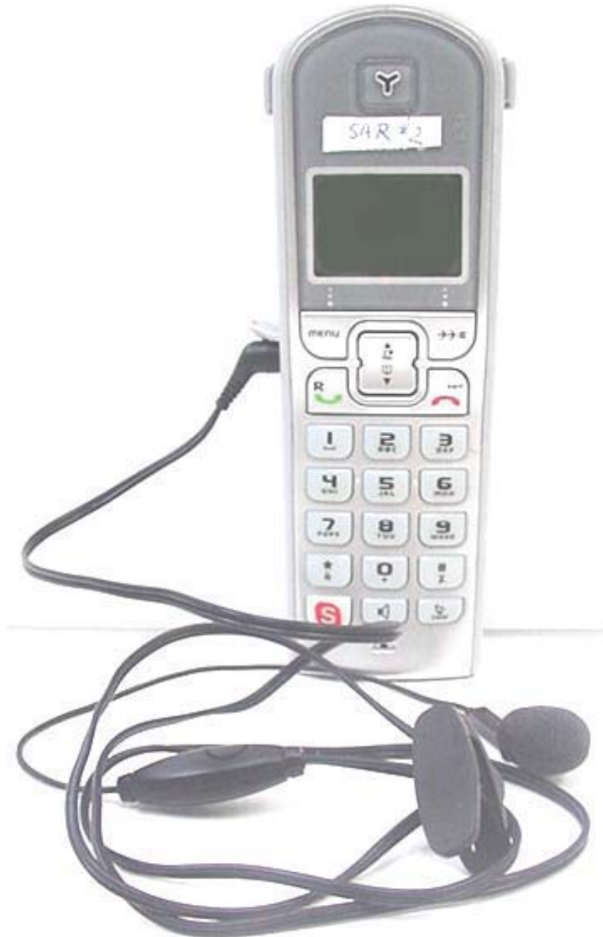
DUT with Generic Ear-Microphone audio accessory
