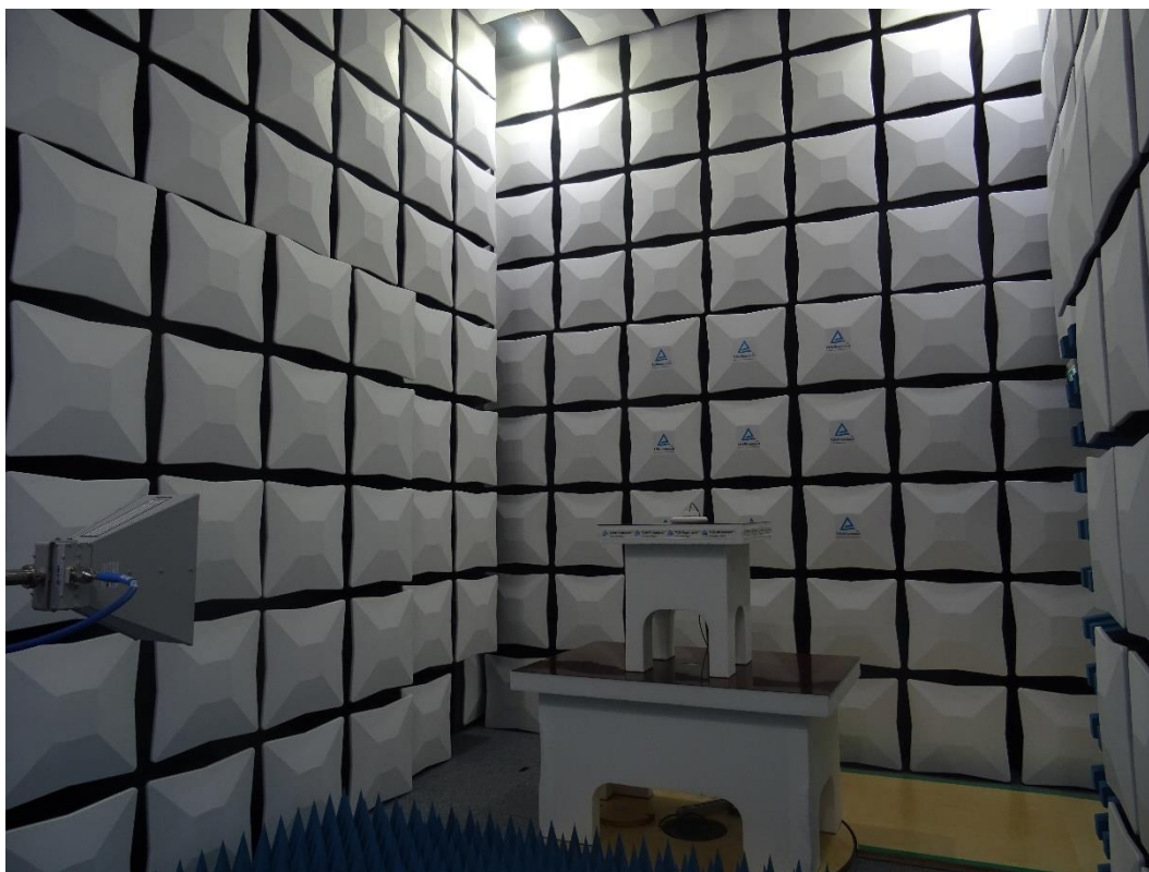
Photo 9: 1GHz to 18GHz - Horizontal polarization
