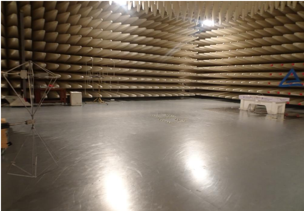
Photo 3: Biconical antenna vertical polarization
