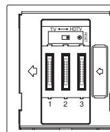
\* To adjust, select the switch located above the song pack slots to HDTV or TV depending on to what kind of TV the device will be connected.
