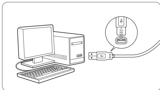
Plug the USB cable to the PC's USB port, as shown in the picture below.
