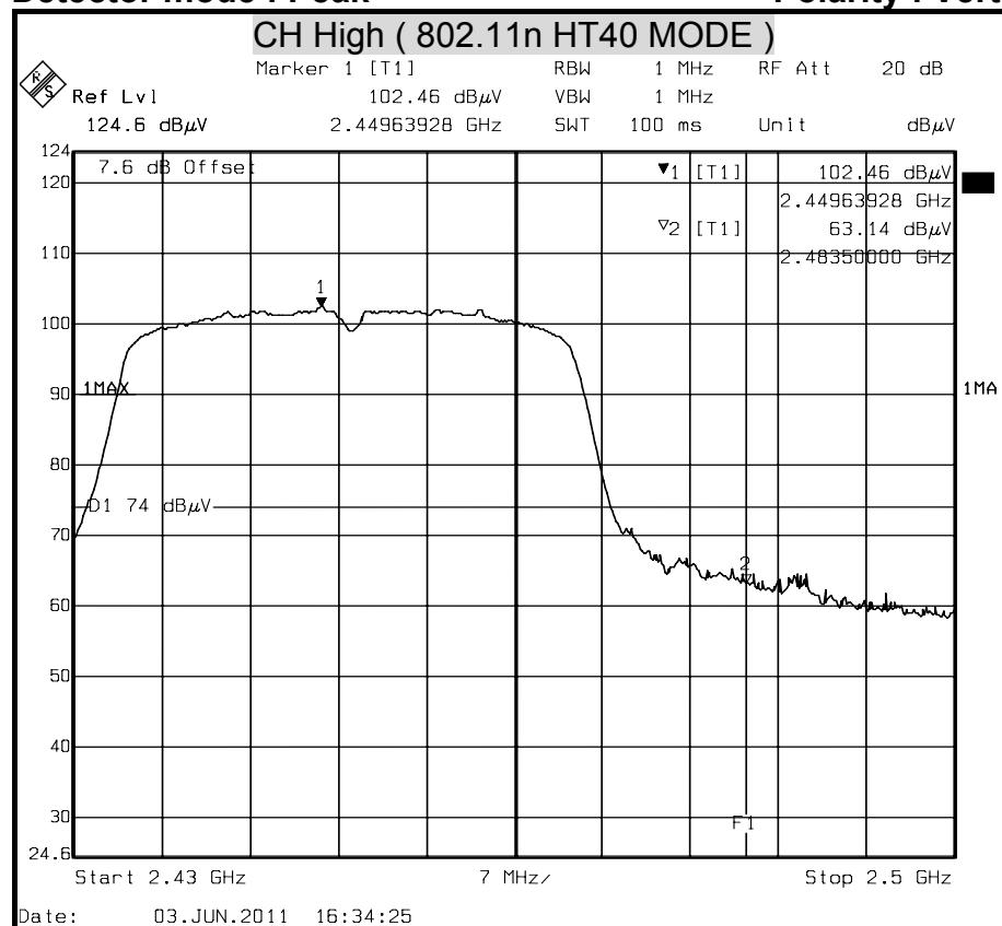
**Detector mode : Average****Polarity : Vertical**
