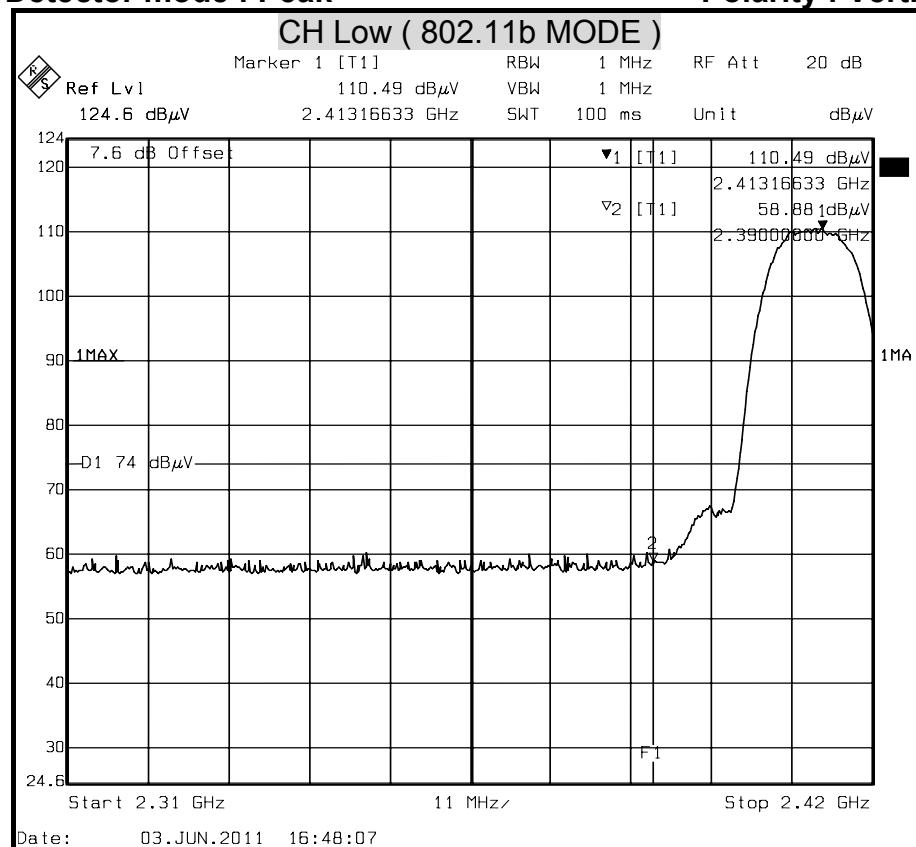
**Detector mode : Average****Polarity : Vertical**
