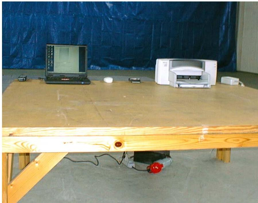
**Test set-up, Radiated Emission**
