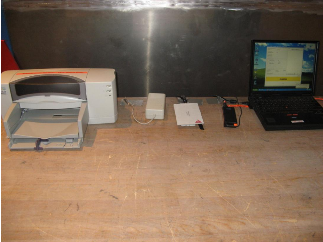
Photo 4.1.1 Test setup regarding measurement of radio frequency voltage on mains.
