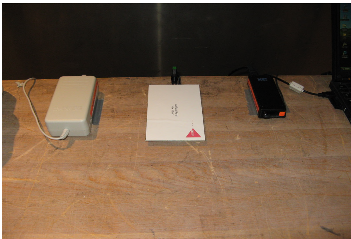
Photo 4.1.2 Test setup regarding measurement of radio frequency voltage on mains with an artificial hand applied to the test object.
