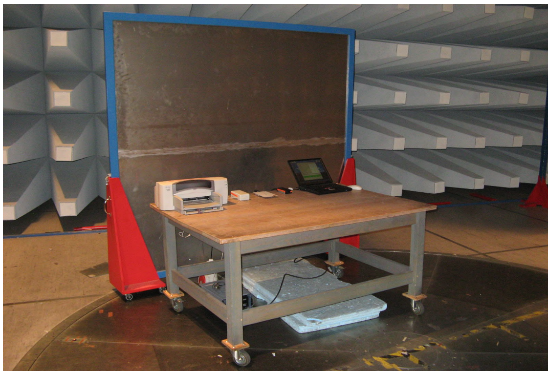
Photo 4.1.1 Test setup regarding measurement of radio frequency voltage on mains.
