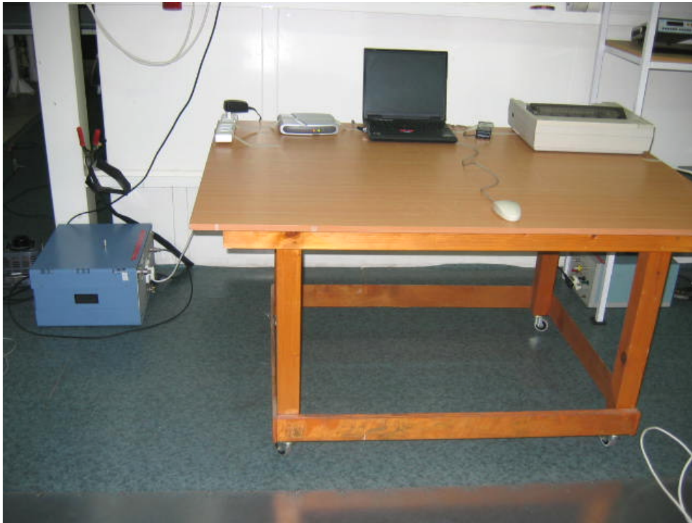
Photograph No.8 Setup for conducted emission measurements at the mains power port
