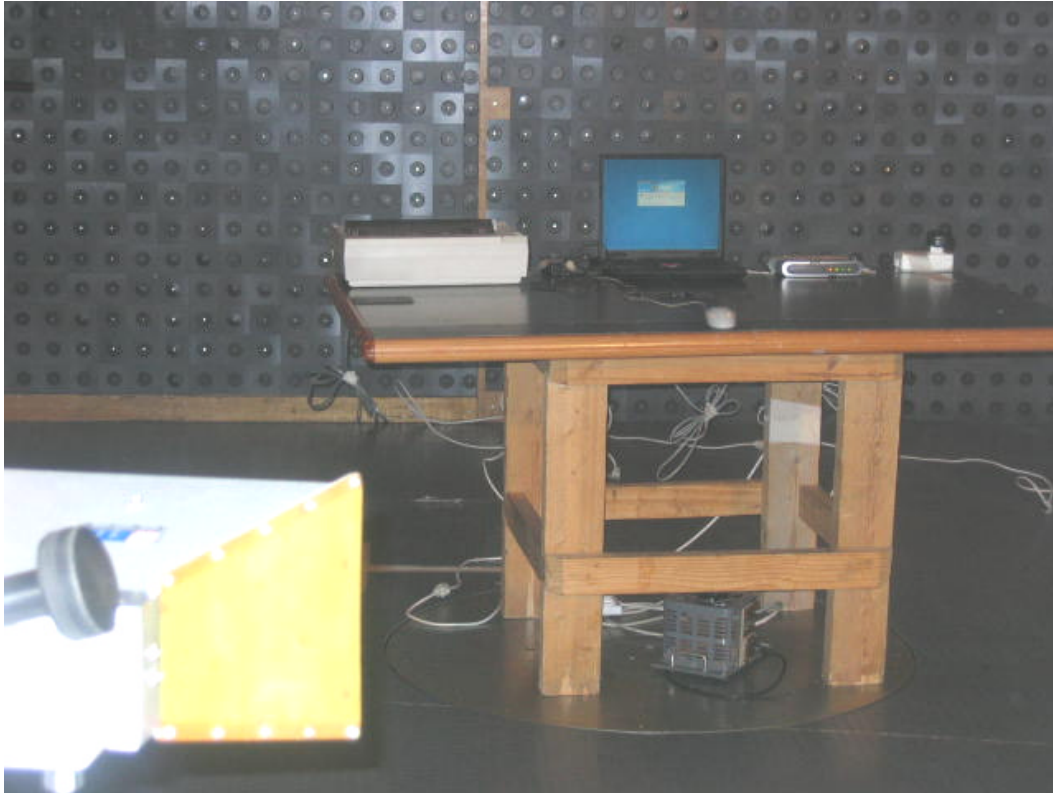
Photograph No.5 Setup for spurious emission field strength measurements above 1 GHz in the anechoic chamber
