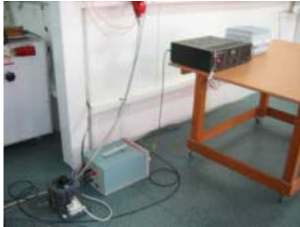
Photograph 8.1.2 Setup for conducted emission measurements at the mains power port
