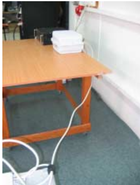
Photograph 8.1.2 Setup for conducted emission measurements at the mains power port
