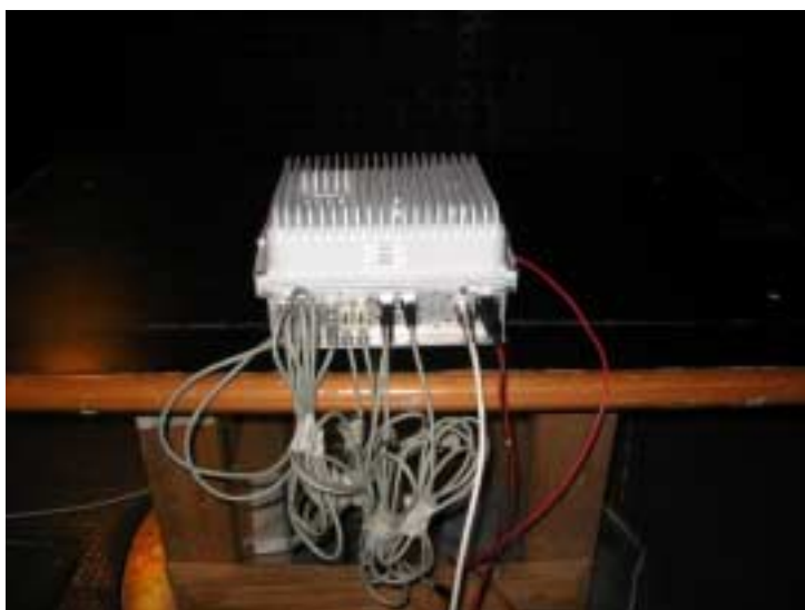
Photograph 7.2.3 Setup for spurious emission field strength measurements in 1 to 8 GHz range at OATS
