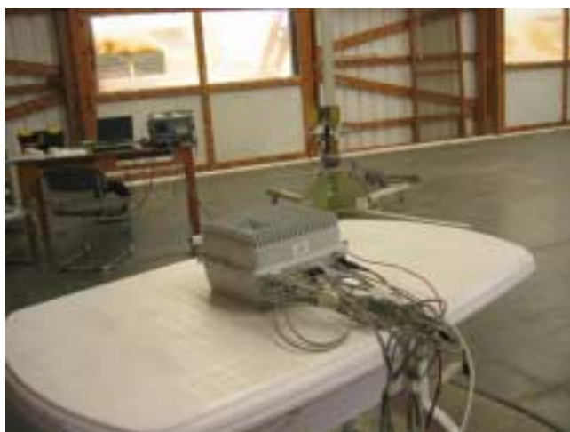
Photograph 7.2.3 Setup for spurious emission field strength measurements in 1 to 8 GHz range at OATS
