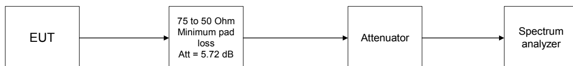
Figure 7.3.1 Spurious emission test setup
