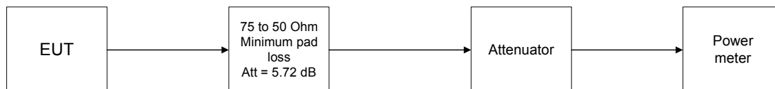
Figure 7.1.1 Peak output power test setup
