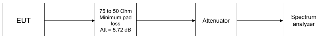
Figure 7.1.1 Peak output power test setup
