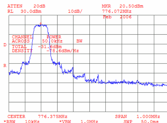
Plot 7.4.6 Adjacent channel coupled power measurements, low carrier frequency, QPSK
