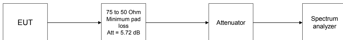
Figure 7.1.1 Peak output power test setup
