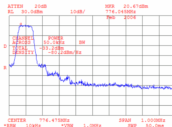
Plot 7.4.8 Adjacent channel coupled power measurements, low carrier frequency, QPSK
