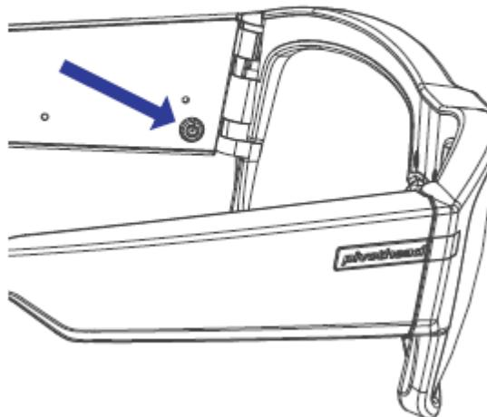
Press power button located inside left temple. Steady blue LED light indicates eyewear is on.
