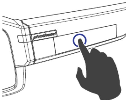
Tap to capture photos. Tap twice to capture burst shots. Tap three times to start/stop a time-lapse.
