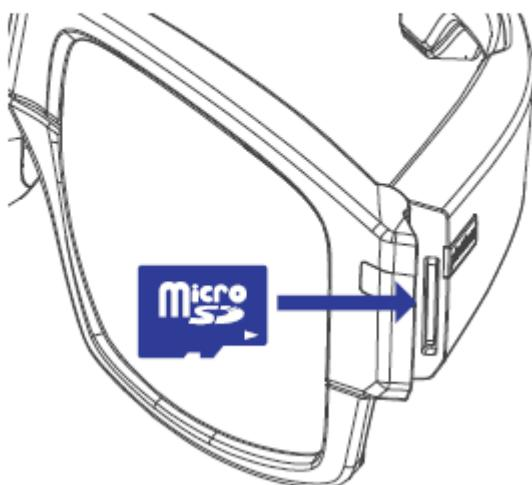
Insert Micro SD card fully into left temple hinge until clicks into place.
