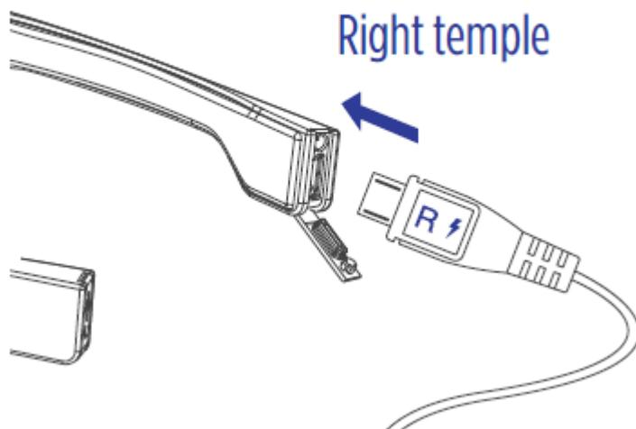
Insert charging cable into right temple. Steady green LED light indicates charging is complete.
