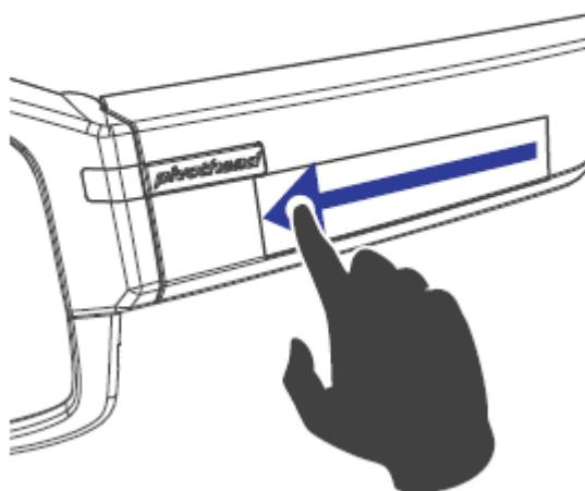
Swipe forward to start a video. Swipe forward again to stop. Flashing red LED light indicates recording.
