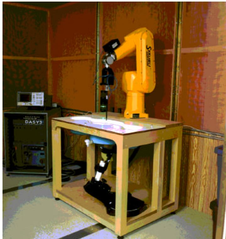
Figure 5. DASY3 SAR Measurement System
