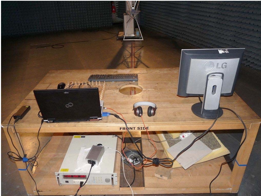
Photo 2: Test setup for radiated measurements (computer peripheral setup, EUT supplied by USB-cable from computer, unintentional radiator S15)
