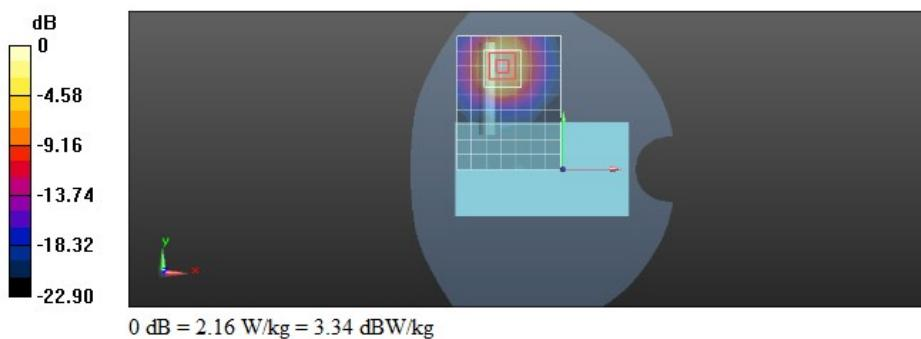
Test Laboratory: CTI SAR Lab
