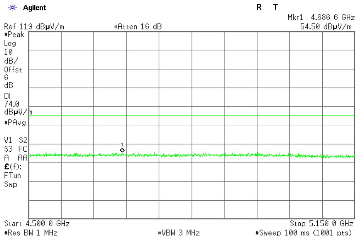
**Detector mode: Average****Polarity: Vertical**
