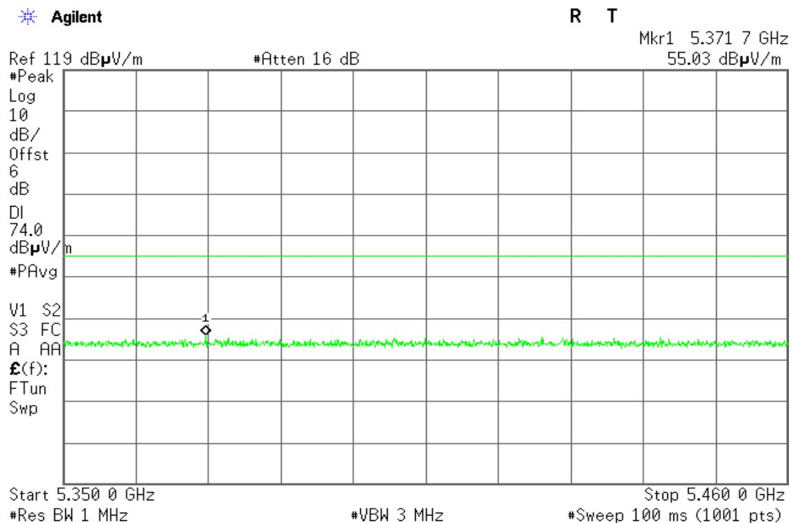
**Detector mode: Average****Polarity: Horizontal**
