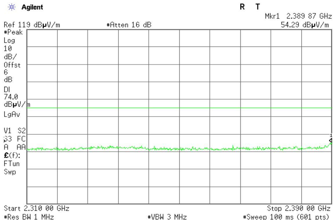
**Detector mode: Average****Polarity: Horizontal**
