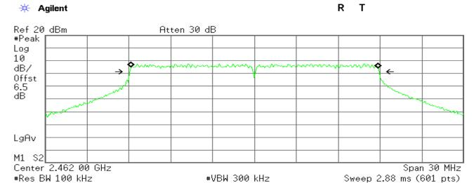
Occupied Bandwidth 17.7254 MHz Occ BW % Pwr 99.00 % x dB -6.00 dB
