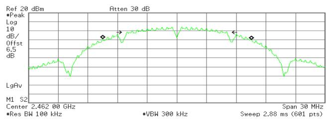
Occupied Bandwidth 15.0656 MHz Occ BW % Pwr 99.00 % × dB -6.00 dB
