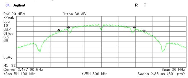
Occupied Bandwidth 15.0636 MHz Occ BW % Pwr 99.00 % x dB -6.00 dB
