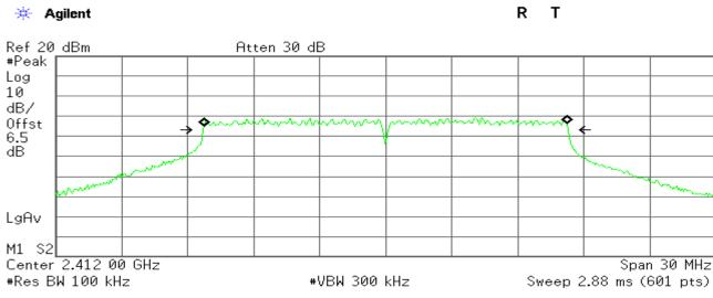
Occupied Bandwidth 16.5142 MHz Occ BW % Pwr 99.00 % x dB -6.00 dB
