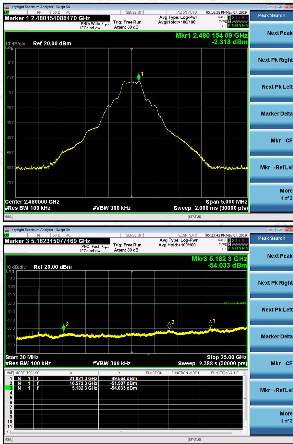
Note: The peak emissions without marker on the above plots are fundamental wave and need not to compare with the limit. The GFSK modulation is the worst case and only those data recorded in the report.
