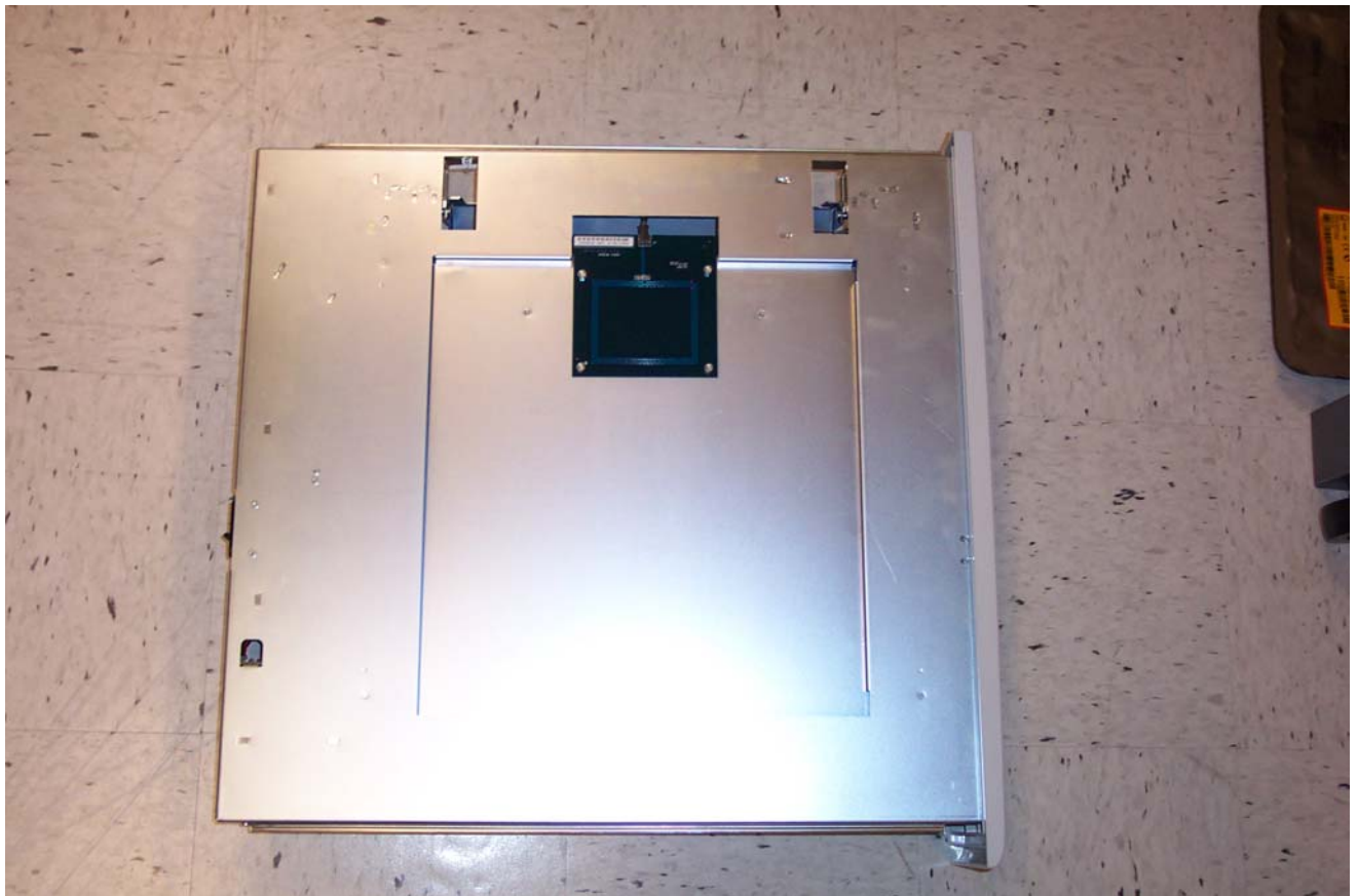
6800 Film Drawer with RF Antenna Bottom
