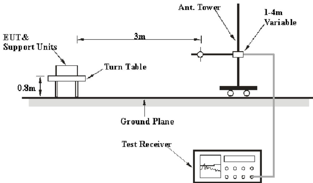
The radiated emission tests were performed in the 3 meters, using the setup accordance with the ANSI C63.4-2003. The specification used was the FCC 15.209 and FCC 15.247 limits.
