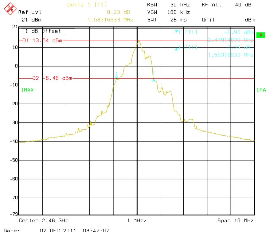
**FCC §15.247(a) (1) (iii)-QUANTITY OF HOPPING CHANNEL TEST****Applicable Standard**
