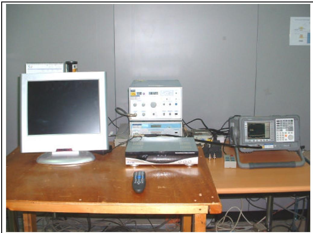
**Test setup photograph for Output Conducted level Emissions.**
