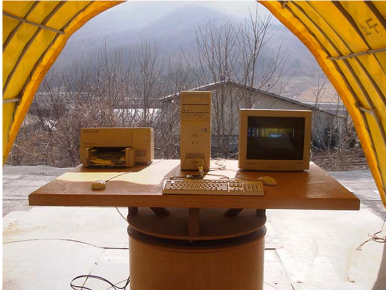
Photograph 1 : Setup for radiated Emissions
