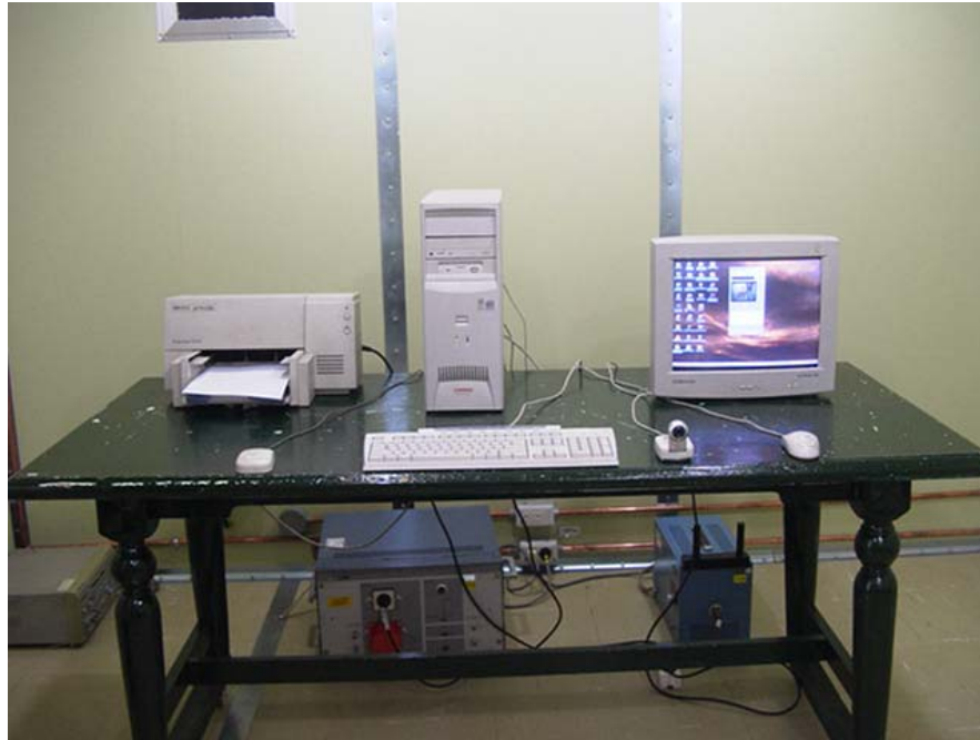
Photograph 2 : Setup for Conducted Emissions
