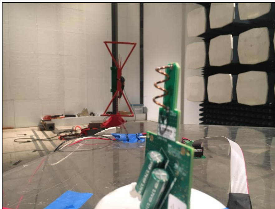
Photograph 1. Radiated Spurious Emissions, Test Setup
