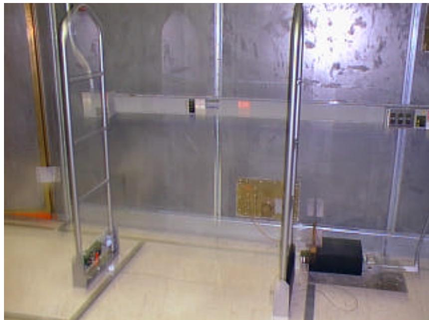
**PHOTOGRAPH 1: CONDUCTED EMISSIONS TEST SETUP**
