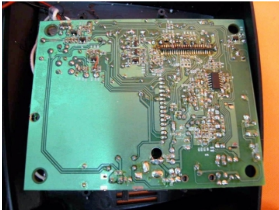
Base Main PCB solder side
