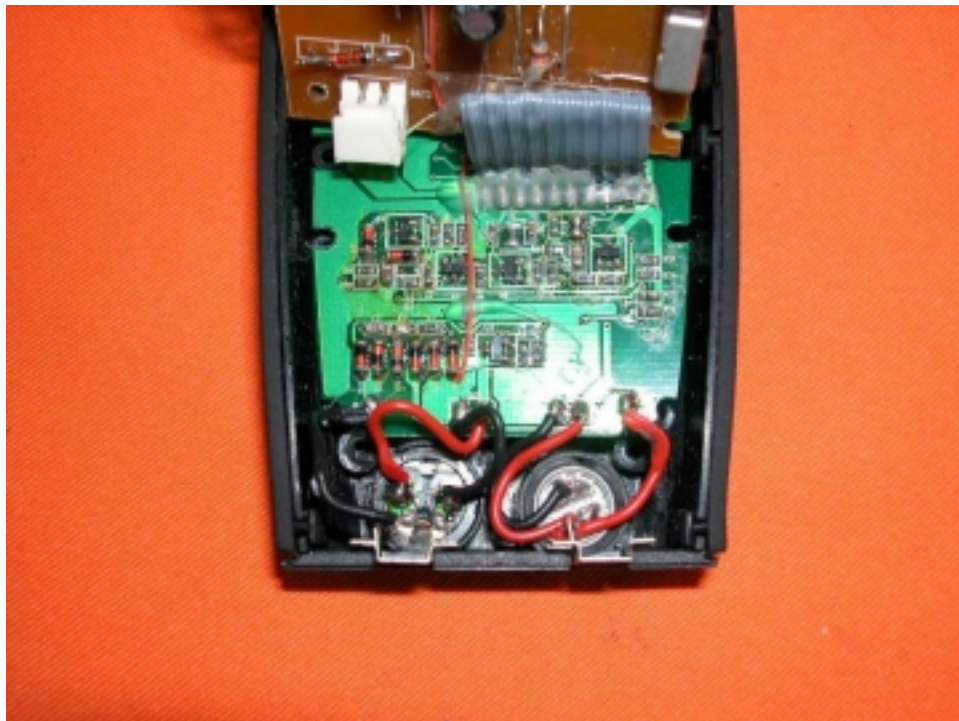
Handset Main PCB comp side (View 3)
