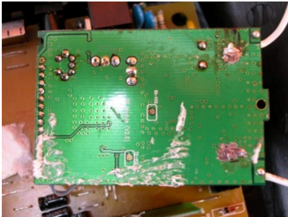
Base Oscillator PCB solder side
