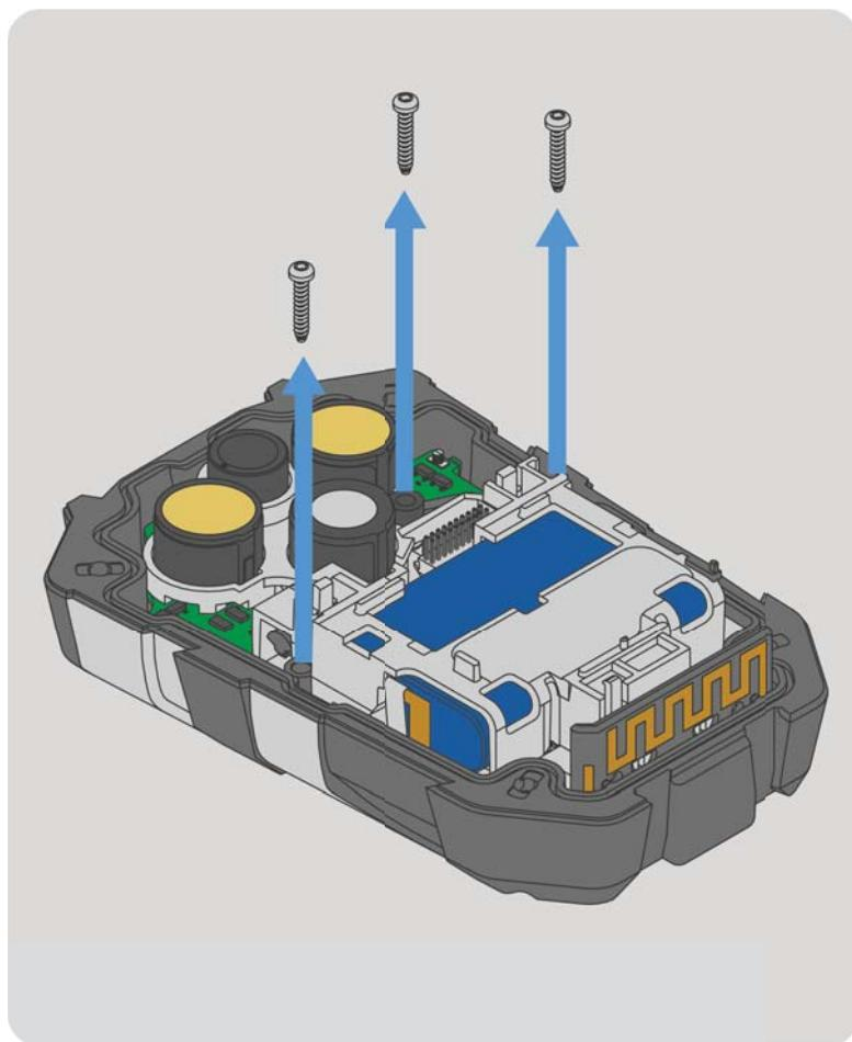
(5) Remove the three internal screws with a Torx T6 screwdriver.
