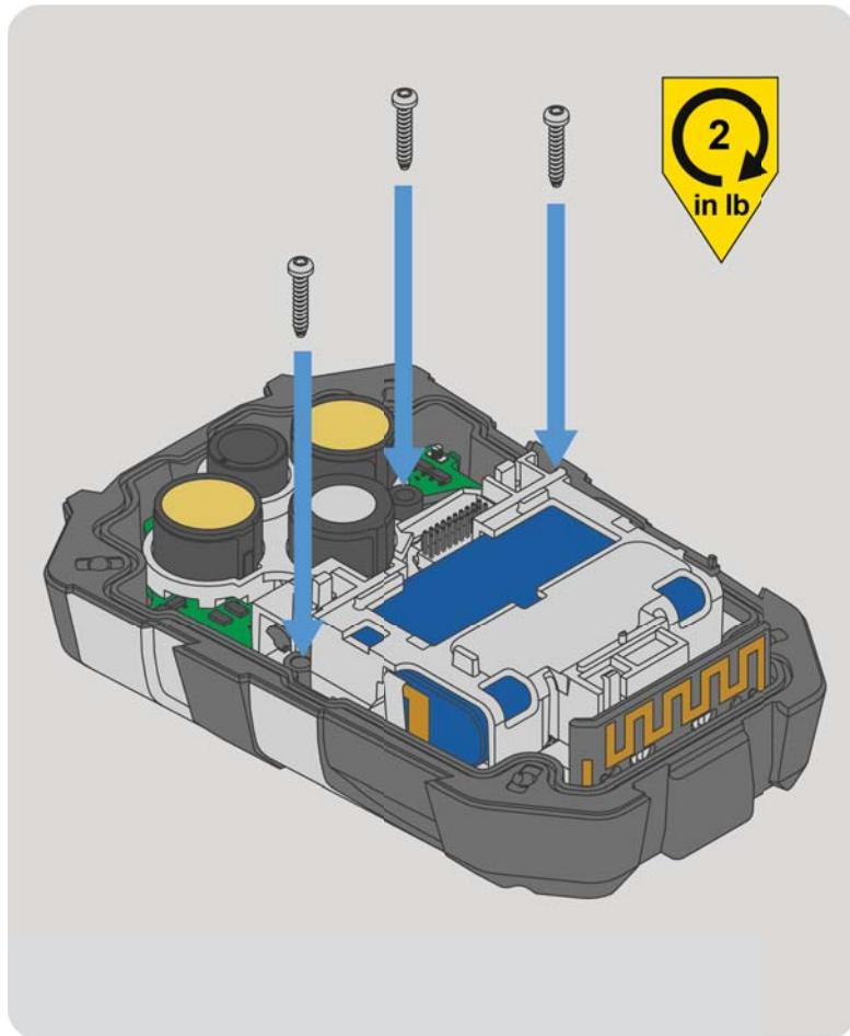
(8) Install the three replacement internal screws with a Torx T6 screwdriver. Torque to 2 in-lbs (0.23 N·m).
