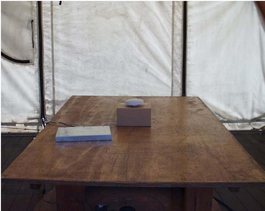
**RADIATED RF MEASUREMENT SETUP WITH BI-DIRECTIONAL ANTENNA**
