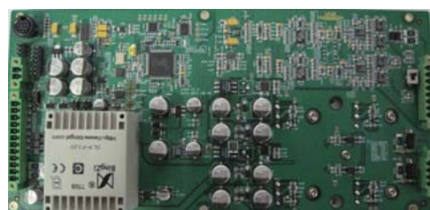
BTL Transceiver PCB ver1.1
