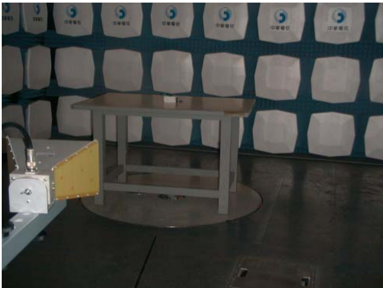
Test Setup for fundamental power
