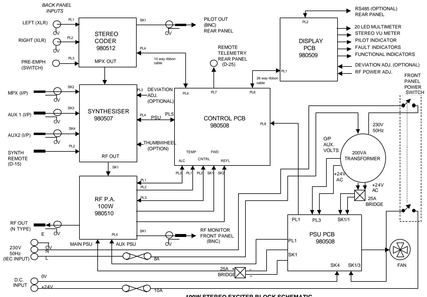
Figure 3: Block diagram of FM-100
