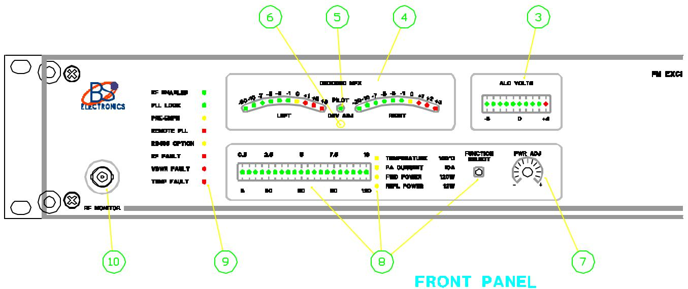
Figure 1: FM-100 Front Panel Controls
