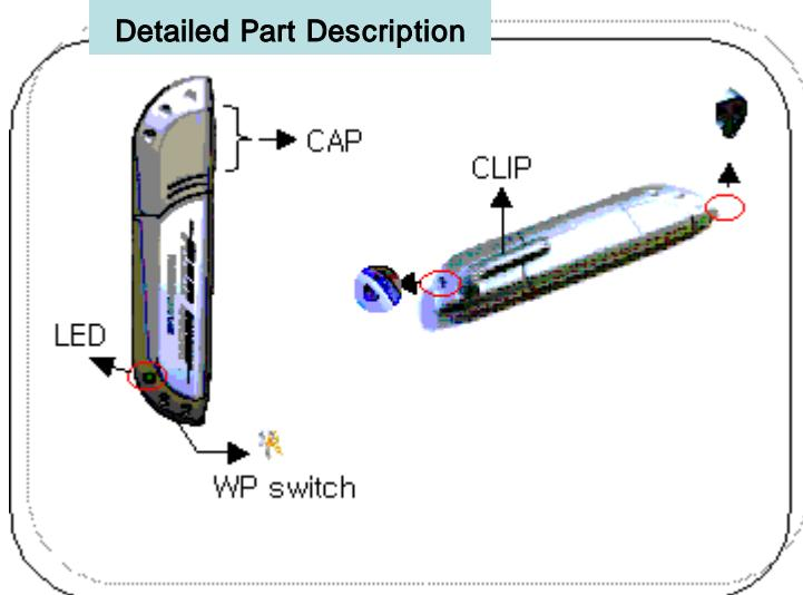
1. Write Protect Switch: To prevent NEXDISK to write, switch to
