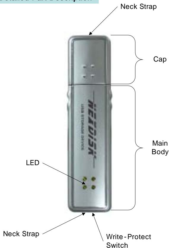
1. Write Protect Switch: To prevent NEXDISK to write, switch to **8**.
