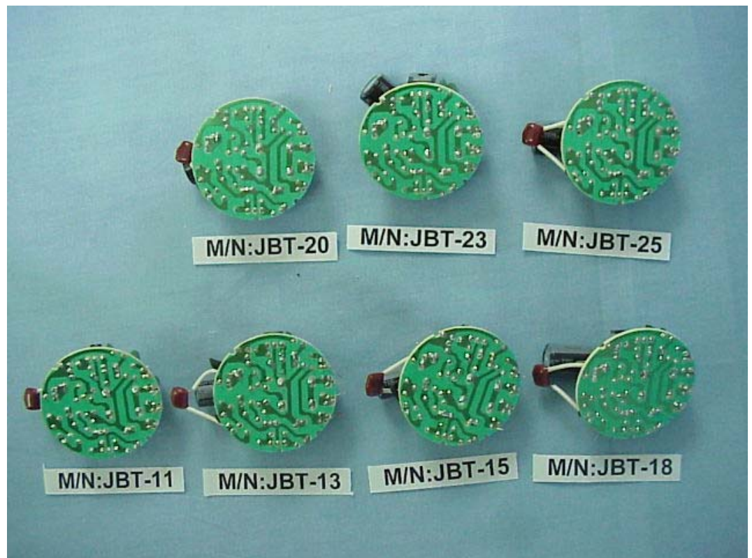
FIGURE 9 ELECTRONIC ENERGY SAVING LAMP (M/N: JBT SERIES) MAIN BOARD (SOLDERED SIDE)
