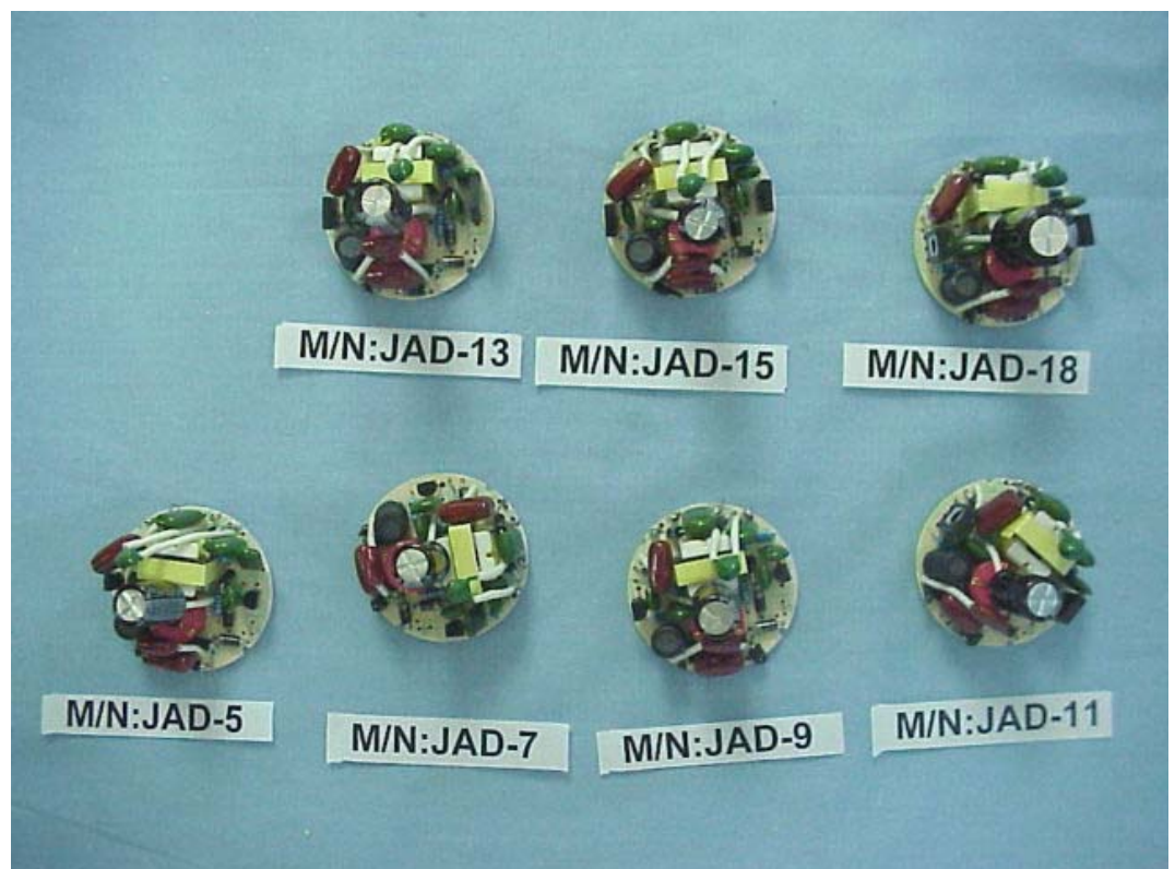
FIGURE 2 ELECTRONIC ENERGY SAVING LAMP (M/N: JAD SERIES) MAIN BOARD (COMPONENT SIDE)
