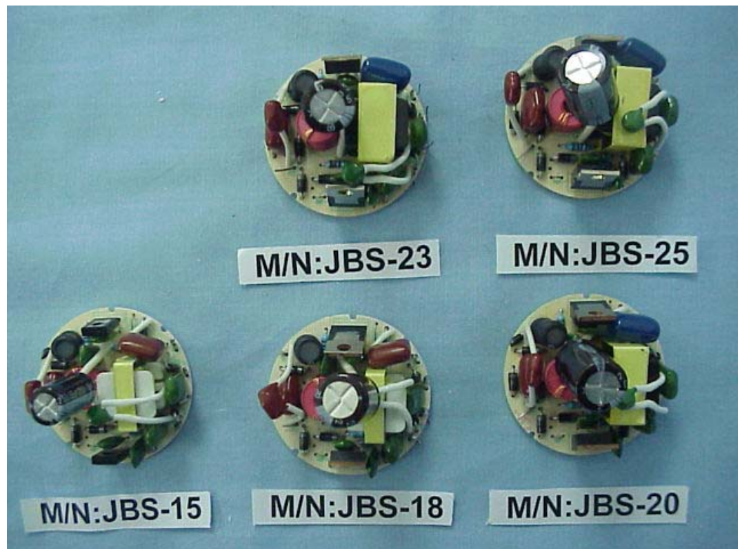
FIGURE 5 ELECTRONIC ENERGY SAVING LAMP (M/N: JBS SERIES) MAIN BOARD (COMPONENT SIDE)
