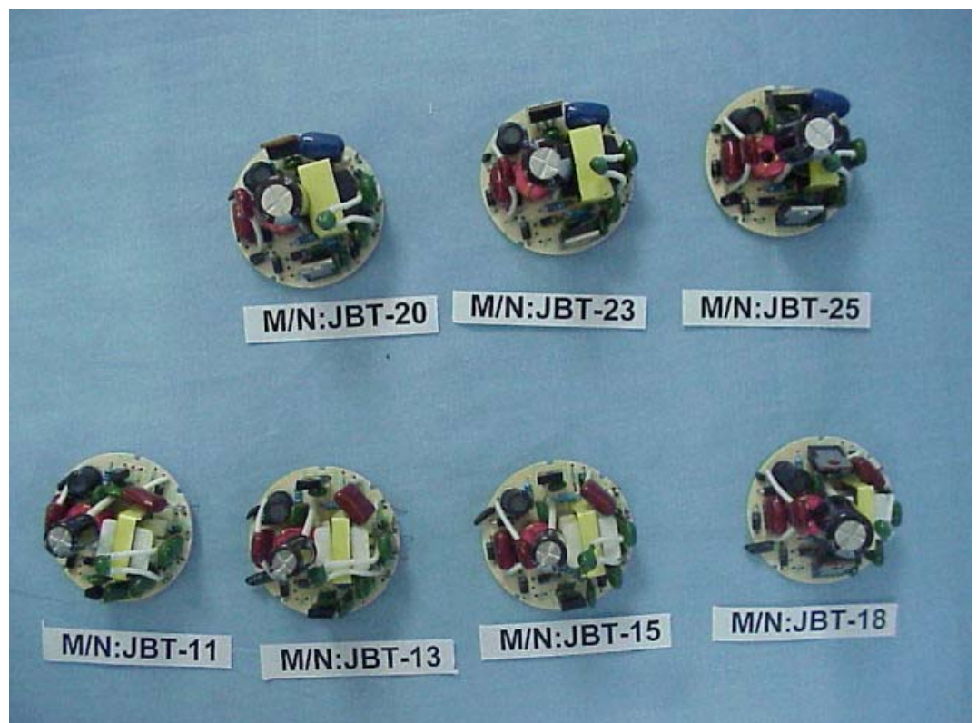
FIGURE 8 ELECTRONIC ENERGY SAVING LAMP (M/N: JBT SERIES) MAIN BOARD (COMPONENT SIDE)
