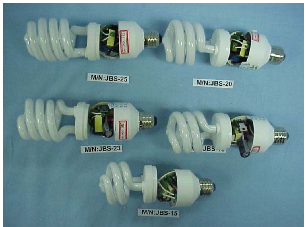
Figure 4 SELF-BALLASTED LAMP (M/N: JBS SERIES) COVER REMOVED
