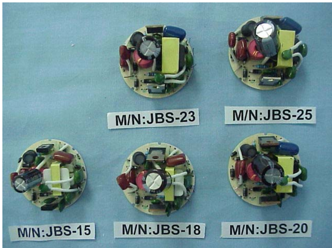
FIGURE 8 ELECTRONIC ENERGY SAVING LAMP (M/N: JBS SERIES) MAIN BOARD (COMPONENT SIDE)
