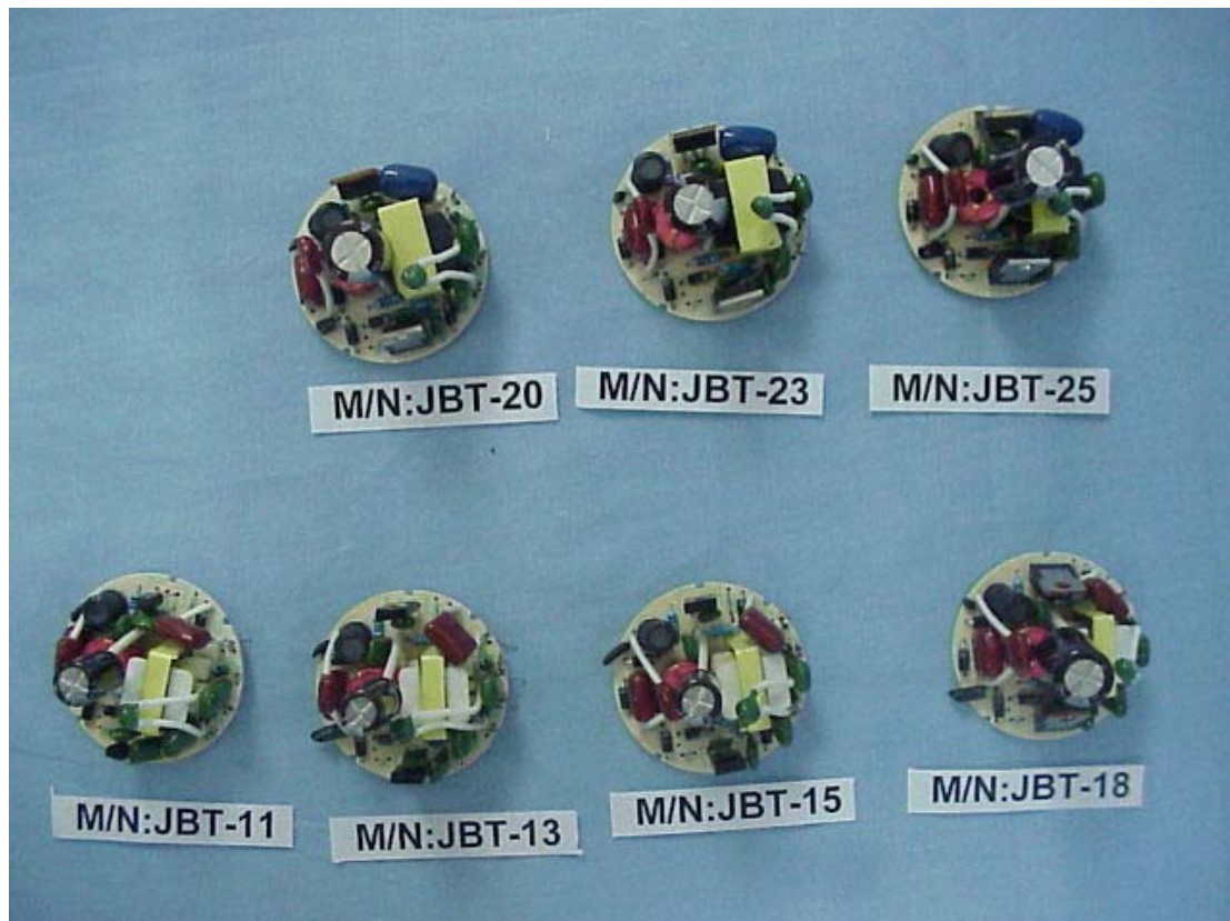
FIGURE 12 ELECTRONIC ENERGY SAVING LAMP (M/N: JBT SERIES) MAIN BOARD (SOLDERED SIDE)
