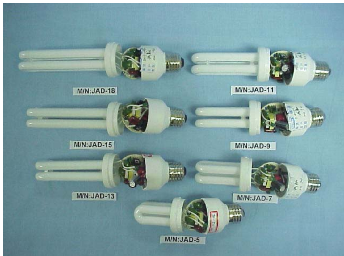
FIGURE 4 SELF-BALLASTED LAMP (M/N: JAD SERIES) COVER REMOVED
