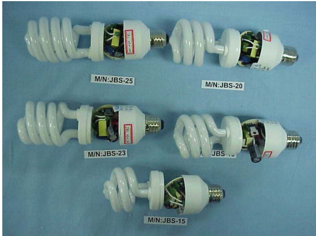
Figure 7 SELF-BALLASTED LAMP (M/N: JBS SERIES) COVER REMOVED
