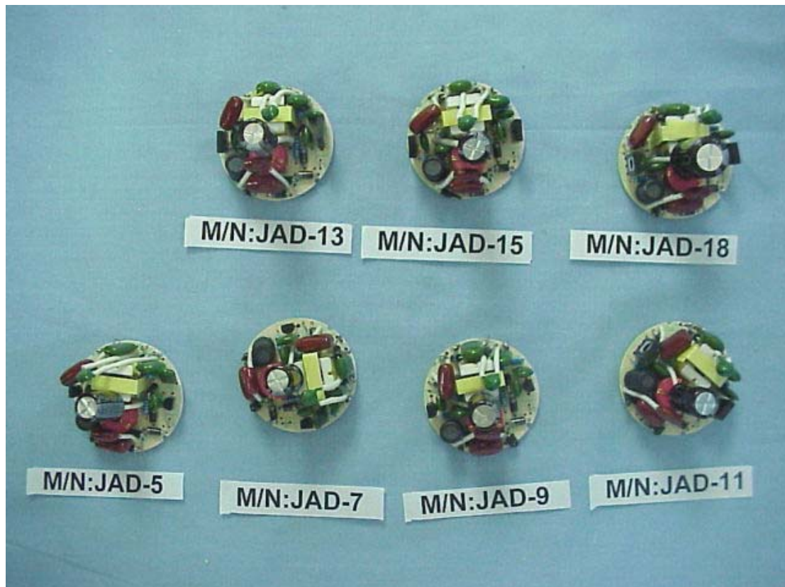
FIGURE 6 ELECTRONIC ENERGY SAVING LAMP (M/N: JAD SERIES) MAIN BOARD (SOLDERED SIDE)
