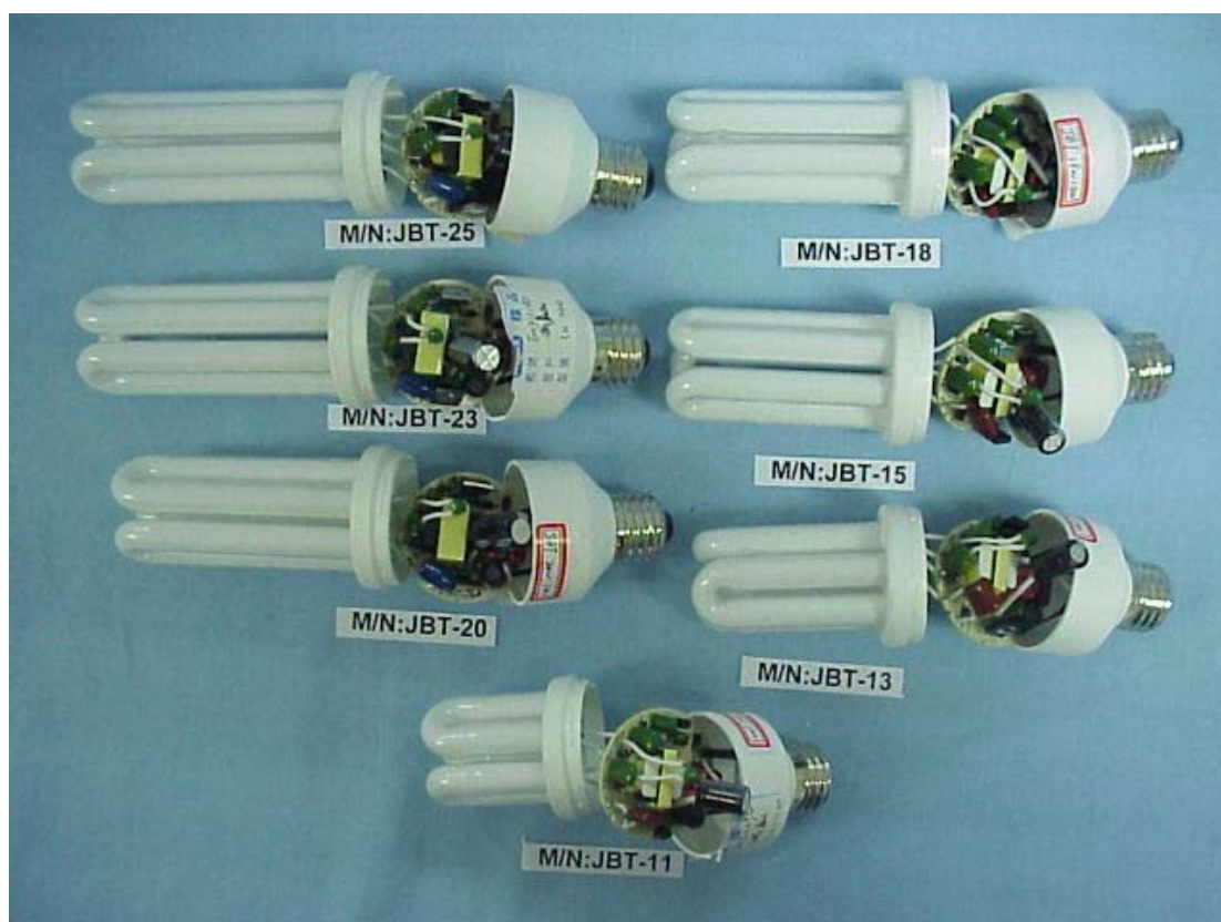
FIGURE 10 SELF-BALLASTED LAMP (M/N: JBT SERIES) COVER REMOVED
