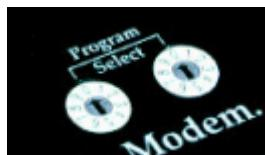
On the XRT Series radios, there is a front panel programming port in addition to the traffic serial port on the rear. Either port can be used for programming, but the above instructions only apply when using the rear traffic port for programming. When using the dedicated front panel programming port, it is not necessary to set the switches to 00 since this connection is only ever used for programming and the radio automatically recognises data on this port as programming data.
