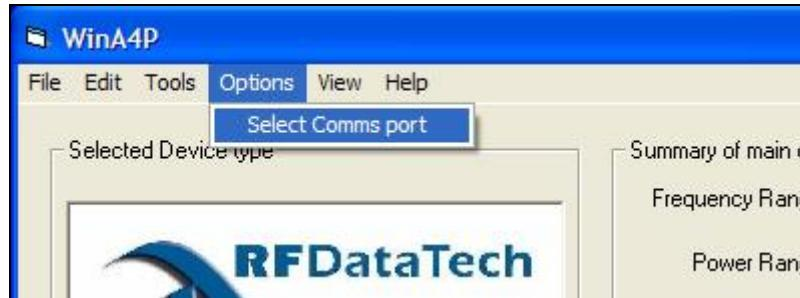
A small sub-window will appear with a pull-down menu allowing selection of port Com 1 to Com 16. Once the required port is selected, press OK to proceed. On most PCs with a single serial port, this port will be Com1.
