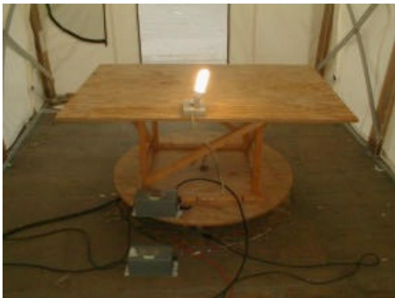
**6.3 Radiated Emission Photograph – Front View (RPW-20E)**
