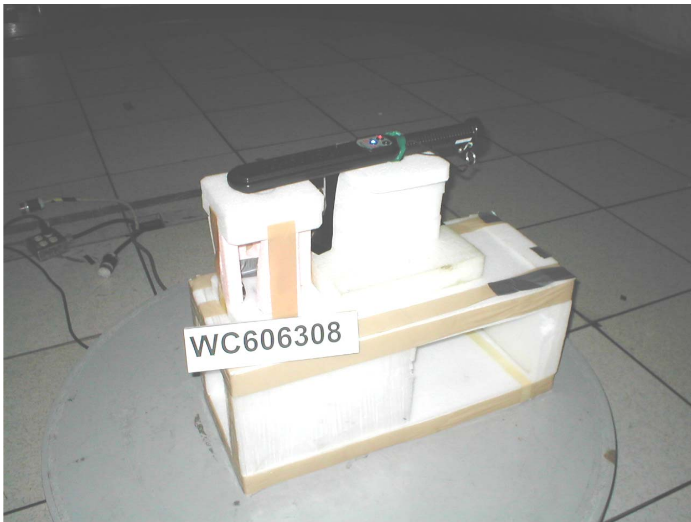
Test-setup photo(s): Radiated emissions test
