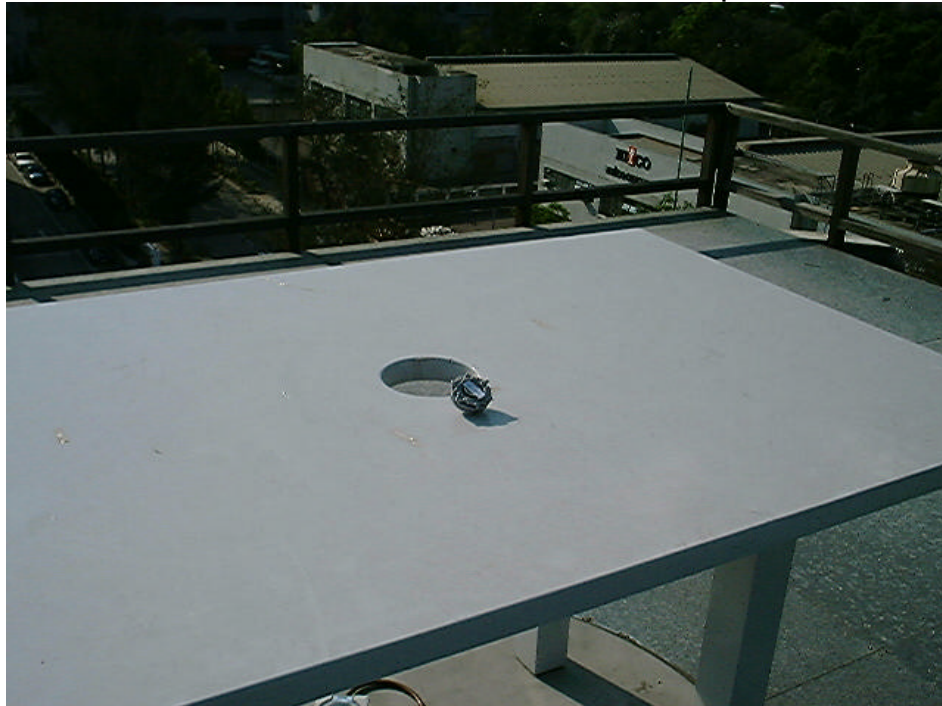
Measurement of Radiated Emission Test Set Up
