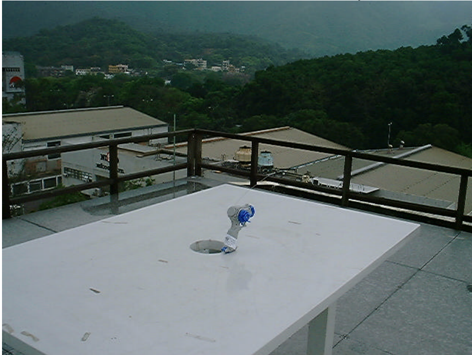
Measurement of Radiated Emission Test Set Up
