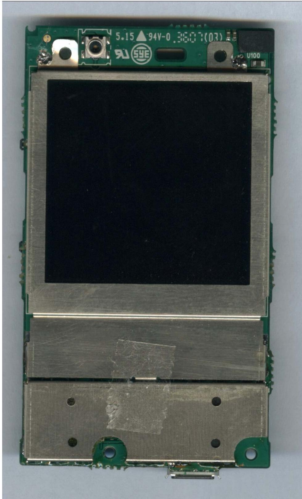
**EUT Internal – PCB Side one, LCD and RF Shielding Removed**
