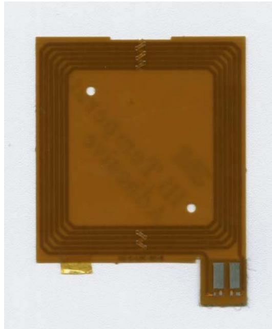
**EUT Internal – GSM 850/1900 Antenna**
